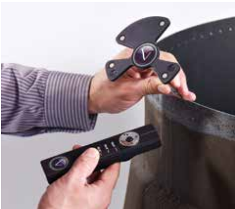
Fast, easy digitizing using a probe to capture points on the part
